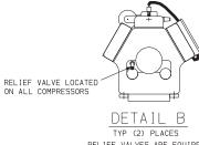
RELIEF VALVES ARE EQUIPPED WITH A 3/8 SAE FLARE FOR FIELD CONNECTION
